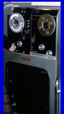
Bottom - Mercury Pool Acoustic Memory Tank Holding 18 mercury delay lines (two views) + UNISERVO tape drive
