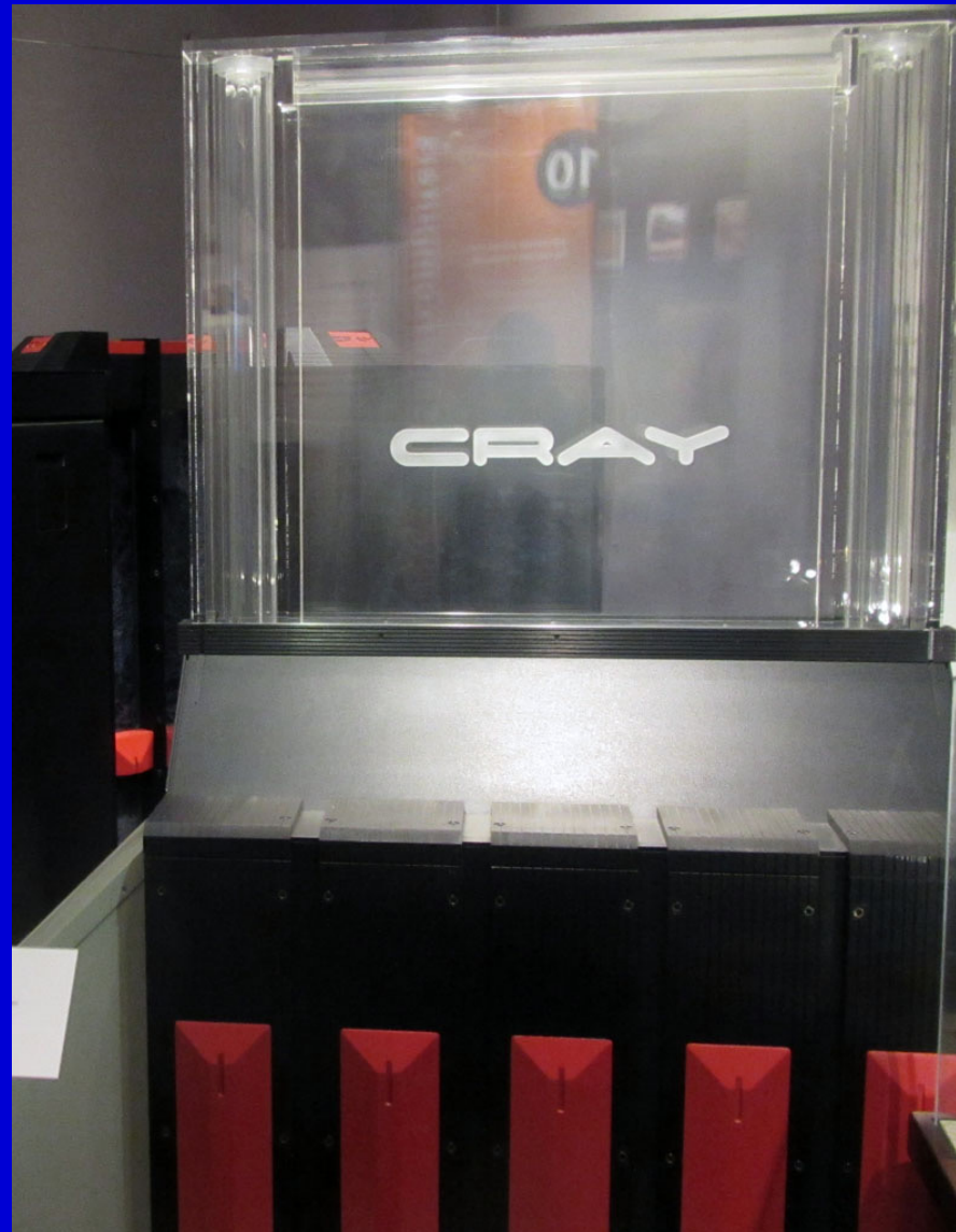
CPU (to left and behind) and Cooling Tower (front)
